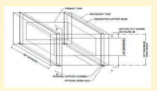
Internal Supported Design (protected tank construction only)
