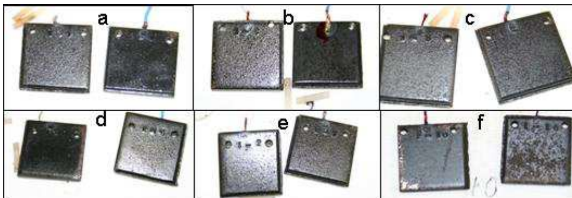
Figure 4. Photographs of carbon steel specimens exposed to ULSD and soy-based biodiesel blends with and without the presence of water: (a) 100% biodiesel, no water added; (b) 50% biodiesel + 50%ULSD, no water added; (c) 100% petroleum diesel, no water added; (d) 100% biodiesel, 1 vol% water added; (e) 50% biodiesel + 50% ULSD, 1 vol% water added and (f) 100% ULSD, 1 vol% water added. Exposure time: 2 months.
