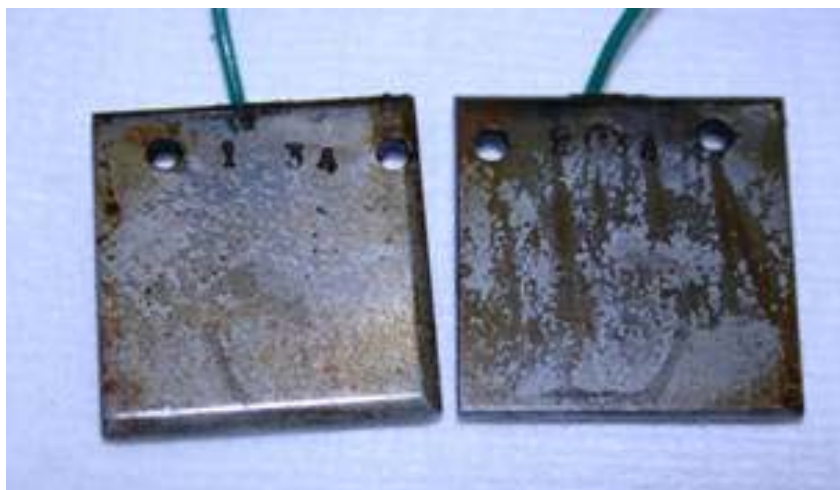
Figure 6. Photographs of carbon steel specimens polished to 600 grit, then exposed to 20% animal-based biodiesel + 80% 4000 ppm S petroleum diesel blend with the presence of 1 vol% water for 3 months.
