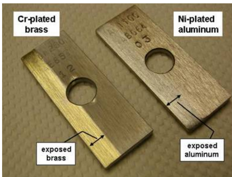
Fig. 3. Appearance of galvanically coupled specimens showing exposed surfaces.
