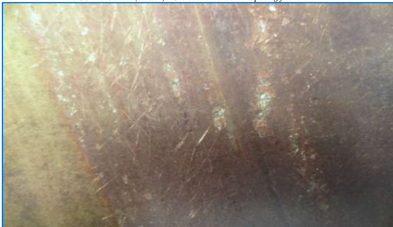
UST 87 Octane (master) - Gel-coat breakdown exposing fibers
