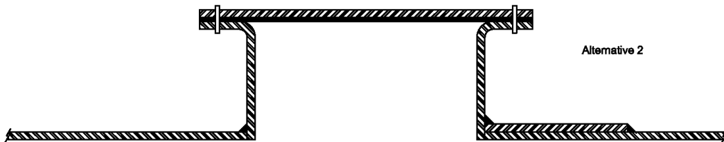
FIGURE 10.4a MANWAY CONSTRUCTION OPTIONS WITH OUTWARD-FACING FLANGE
