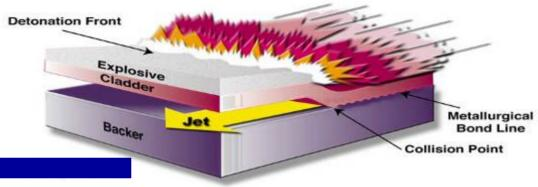
Cladding and Base Metal Plates are positioned parallel with a preset separation distance.
