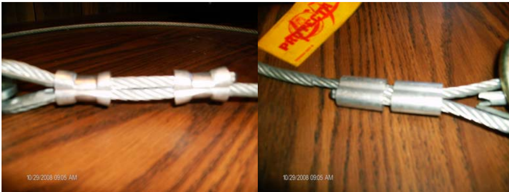
Properly crimped fittings at one end.
