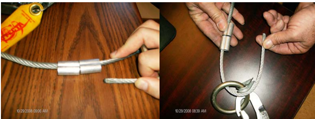
Wire rope pulls free of fittings with minimal force applied.
