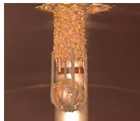
Corrosion on fittings in an FRP tank (left) and a steel tank (right). Both tanks store ULSD.
