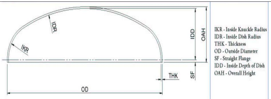
2:1  $\rightarrow$  IKR IS APPROX 15% OF DIA – IDR IS APPROX 80% OF DIA 90/17  $\rightarrow$  IDR IS 90% OF DIA - IKR IS 17% OF DIA (Accepted by Code) IDD  $\rightarrow$  ID / 4
