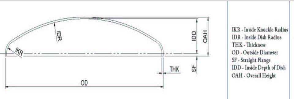
IKR MUST BE A MINIMUM 6% OF DIAMETER (OR 3 x THICKNESS IF GREATER)
