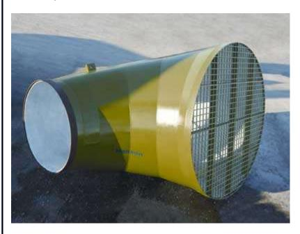
The unique requirements of Juliff Pump Station No. 1 in Fort Bend County, Texas included rotation and welding together the five segments to create an 87.8-degree bend. The fittings – completed in 2007, but due for installation this year – will enable the pump station to withdraw water from the Brazos River.
