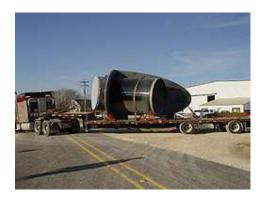
Among Pipe entries, the winner was a unique discharge pipe created for the Waxahachie Pump Station of the Tarrant Regional Water District in Fort Worth, Texas. RTLC Piping Products of Kosse, Texas fabricated the pipe with a cement-mortar lining and polyurethane coating. The discharge pipe featured four-inch-thick (101.6 millimeters) reinforcing plates to withstand the 250 pounds per square inch (17.58 kilograms per centimeter) design pressure.
