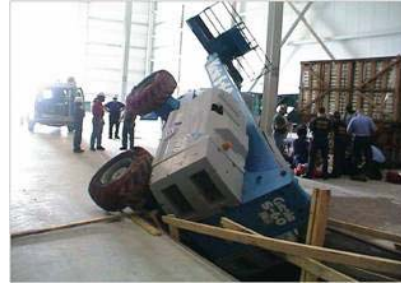
Tipovers are the most common aerial lift accident
