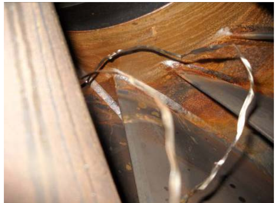
42" Gasket inner ring stuck in 1 st stage impeller
