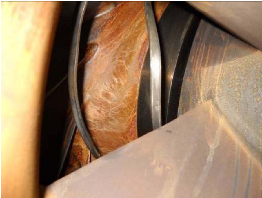
42" Gasket inner ring stuck in 1 st stage impeller
