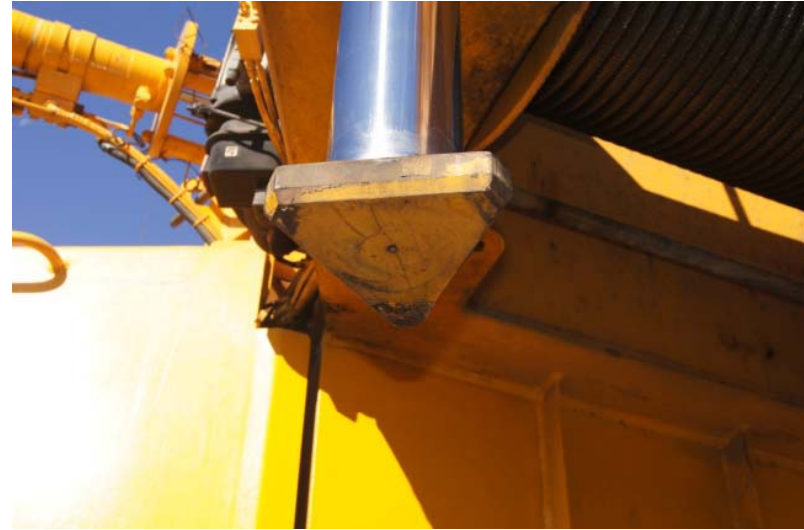
Close up view of hydraulic ram at south side of crane. End triangular locking piece intact
