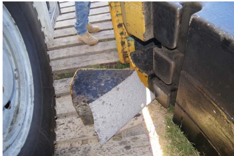
Piece of counterweight broke from main assembly during incident
