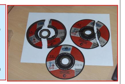
**Disc Information:** Tyrolit 5" Cutting Discs used on standard grinding machine @ 8800RPM The maximum advised disc speed is 12,225 RPM. The discs were used to cut carbon steel material.
