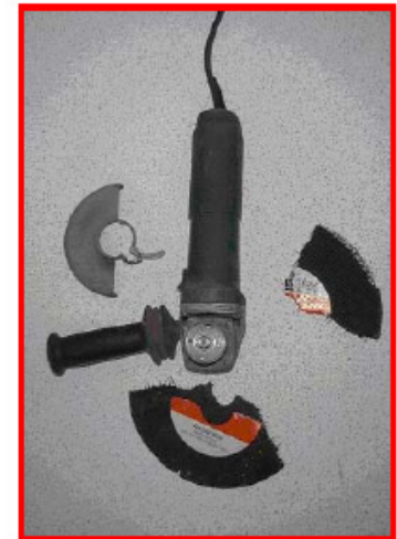
Angle grinder and disintegrated disk
