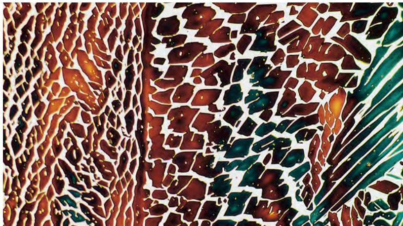
Metallographic structure of 2205 duplex weld metal, 500x (Source: Lincoln Smitweld bv)
