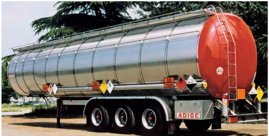
Lean duplex stainless steel asphalt hauling tanker (Source: Outokumpu)
