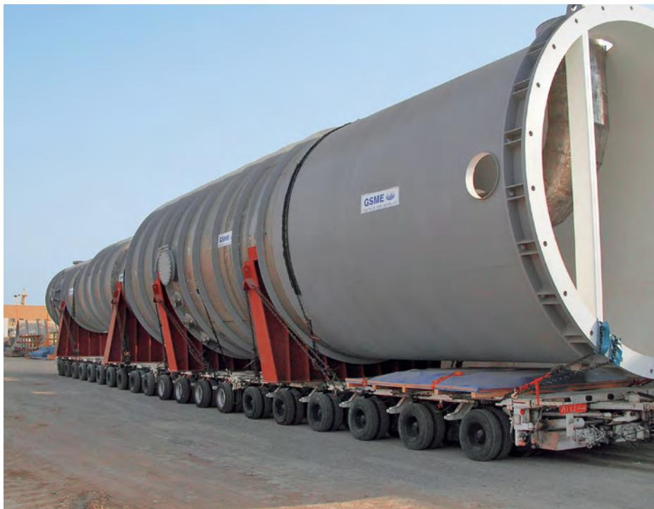
2507 stainless steel falling film evaporator (Source: Gary Carinci, TMR Stainless)
