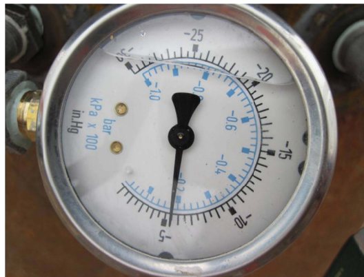
Picture 7 - Gage Reading at UL 1316 Test Requirement
