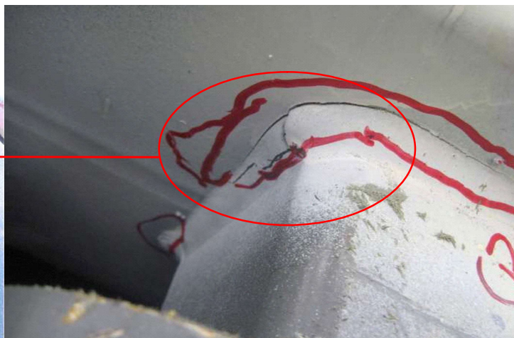
Results of NDT on another unit showing failure point in same location
